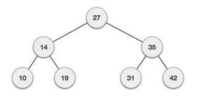
We observe that the root node key (27) has all less-valued keys on the left subtree and the higher valued keys on the right sub-tree.
