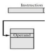
**Absolute mode:** The operand is in a memory location; the address of the operand is passed explicitly in the instruction. Global variables are represented using this addressing mode.
