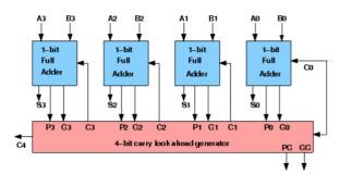
The number of gate levels for the carry propagation can be found from the circuit of full adder. The signal from input carry  $C_{in}$  to output carry  $C_{out}$  requires an AND gate and an OR gate, which constitutes two gate levels. So if there are four full adders in the parallel adder, the output carry  $C_5$ would have 2 X 4 = 8 gate levels from  $C_1$  to  $C_5$ . For an n-bit parallel adder, there are 2n gate levels to propagate through.
