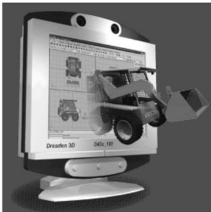
Active auto-stereoscopic 3-D Display (courtesy of Dresden 3D Co.)
