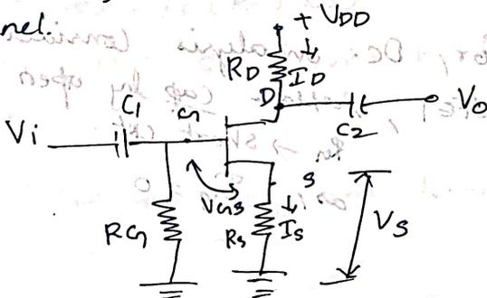
Now  $V_{GS} \rightarrow$  controlling  $V_{GS}$  is determined by volt across  $R_S$
