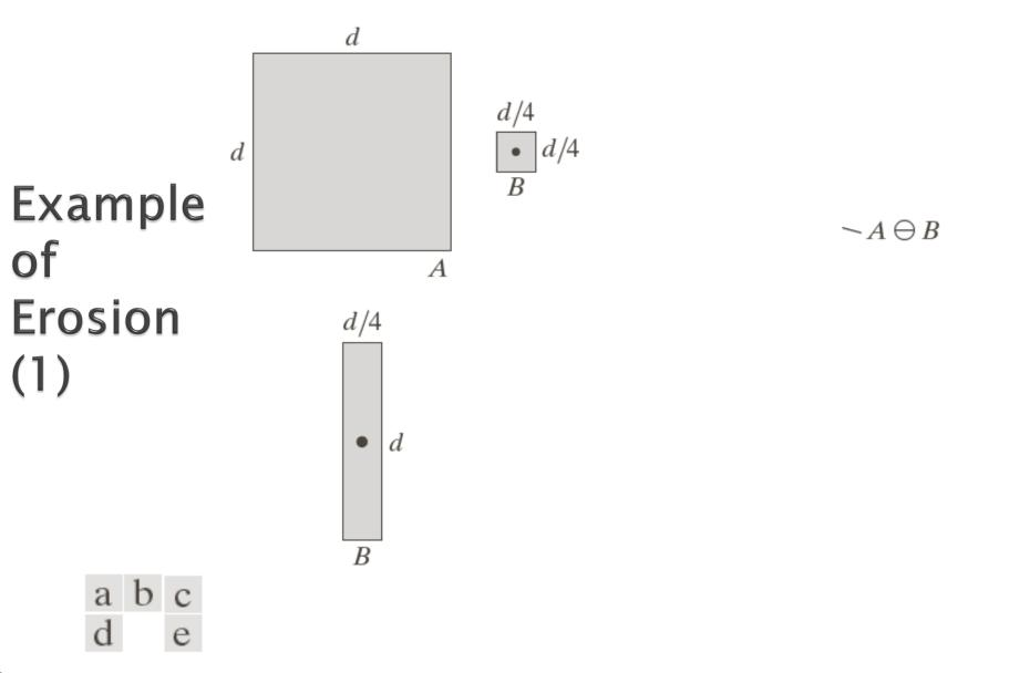
**FIGURE 9.4** (a) Set A. (b) Square structuring element, B. (c) Erosion of A by B, shown shaded. (d) Elongated structuring element. (e) Erosion of A by B using this element. The dotted border in (c) and (e) is the boundary of set A, shown only for reference.
