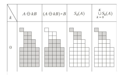
**FIGURE 9.24** Implementation of Eqs. (9.5-11) through (9.5-15). The original set is at the top left, and its morphological skeleton is at the bottom of the fourth column. The reconstructed set is at the bottom of the sixth column.
