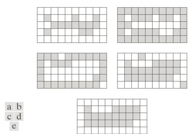
**FIGURE 9.22** (a) Set A. (b) Complement of A. (c) Result of thinning the complement of A. (d) Thickened set obtained by complementing (c). (e) Final result, with no disconnected points.
