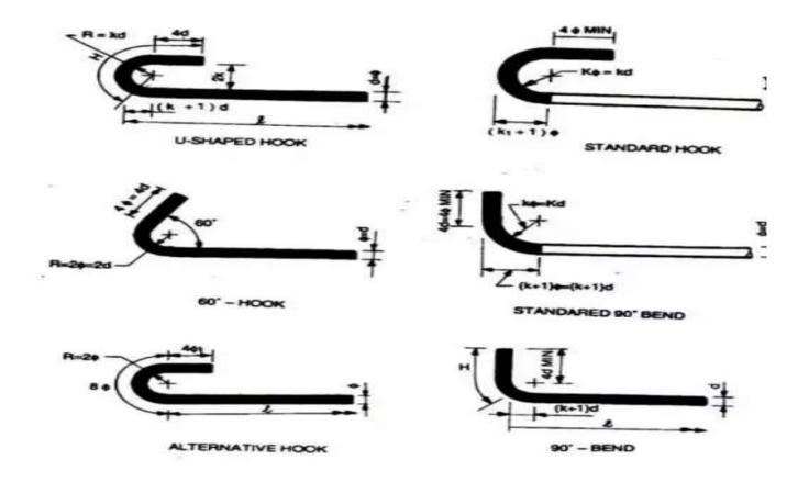
Fig.1: Standard Hooks and Bends in Reinforcement
