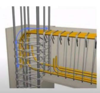
Length of steel bar needed to be embedded into the column to establish the desired bond strength between concrete and steel
