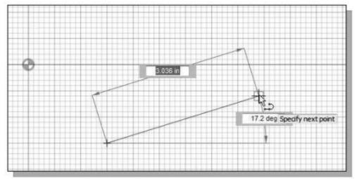
3. Move the graphics cursor toward the right side of the graphics window and create a horizontal line as shown below (Point 2). Notice the geometric constraint symbol, a short horizontal line indicating the geometric property, is displayed.
