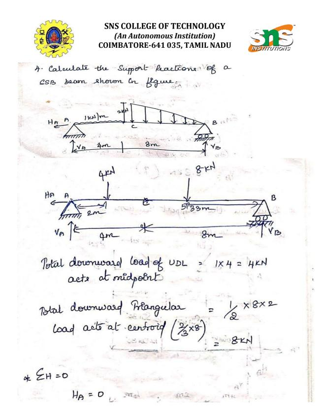
**SNS COLLEGE OF TECHNOLOGY** (An Autonomous Institution) **COIMBATORE-641 035, TAMIL NADU** & EV=D VA+YB - (1×4) - (1/2×8×2) ZD VB+VB-4-8 (2) = 0 VA+VB= 12 -EMA= D (4×2) + (8×(12-5:33) - VB×12 = 0. 12 VB = 8+53.36 VB = 5,11 KN Sub VB En D VA+VB=12 6.8KN
