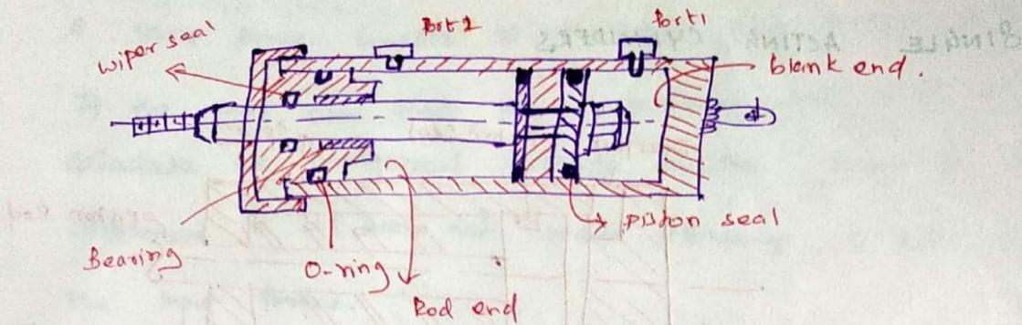
\* A double acting cylinder capable of delivering forces in both directions. The barrel is made of seamless steel tubing, honed to a fine finish on the inside surface.
