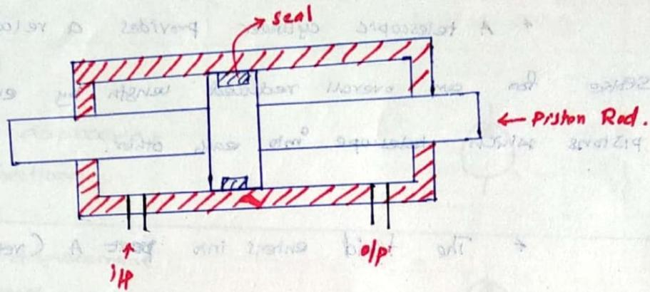
Double rod cylinder is a cylinder with a single piston and a piston rod extending from each end. This cylinder allows work to be performed at either (or) both ends. It may be desirable where operating speed and return speed are equal.
