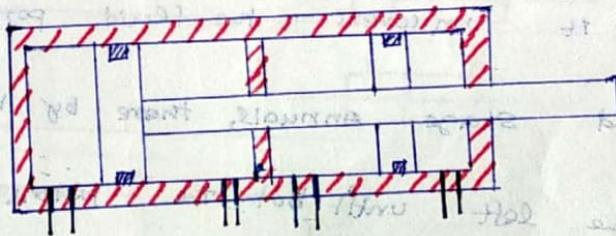
Tandem cylinder design has two cylinders mounted in line with position connected by a common piston rod. These cylinders provide increased output force when the bore size of a cylinder is limited. But the length of the cylinder is more than a std cylinder and also requires a larger flow rate to achieve a speed because flow must go to both pistons.
