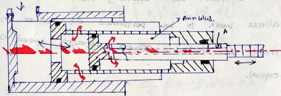
The first stage piston is forced to the left until it uncovers the fluid ports connecting this with the second stage annulus, there by moving the larger piston to the left until both the pistons are fully retracted into the body of the cylinder.
