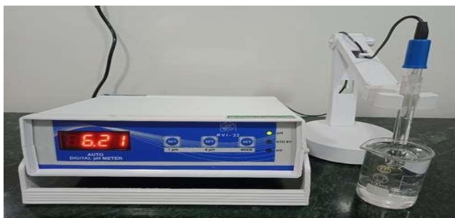
Figure 1: The pH meter with glass membrane electrode.
