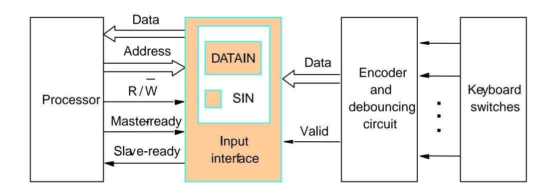
•*Keyboard is connected to a processor using a parallel port.* •*Processor is 32-bits and uses memory-mapped I/O and the asynchronous bus* protocol.
