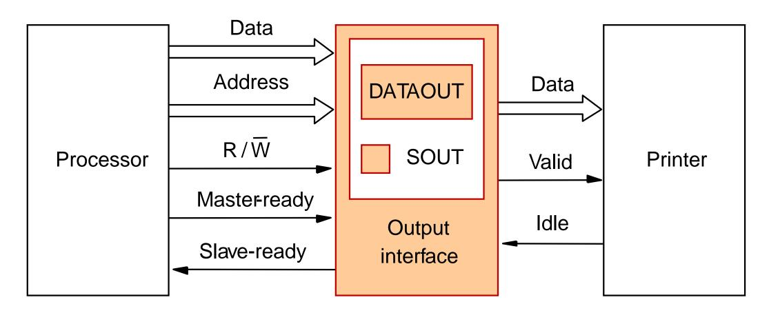
•*Printer is connected to a processor using a parallel port.* •*Processor is 32 bits, uses memory-mapped I/O and asynchronous bus protocol.*
