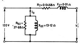
(ii) Output =  $50,00 \times 0.8 = 40,00$  W ;  $I_{2(f.1)} = 50,000/120 = 416.67$  V ; copper losses,  $W_c = (I_{2(f.1.)})^2 \times R_2 = (416.67)^2 \times 0.00468 = 812.5$  W.
