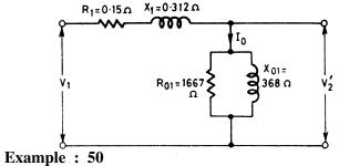
A 50 kVA, 1,000/200 V, 1-phase, step-down transformer takes 4 A at p.f. of 0.2 lagging. When the secondary is open-circuit. Calculate the primary current, and p.f., when a load taking 250 A at a lagging p.f. of 0.8 is connected across the secondary. Assume the voltage drop in the winding to be negligible.
