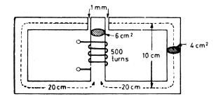
Thr cross-section of central limb is 6 cm2, and of each outer limb is 4 cm2. If the coil is wound with 500 turns, calculate the exciting current required to set up a flux of 0.9 mWb in the central limb. B-H curve of wrought iron are :
