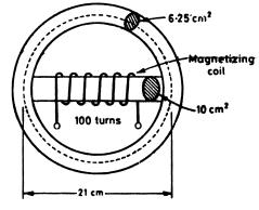
Here  $\phi = 1.25 \text{ mWb} = 1.25 \times 10^{-3} \text{ Wb}$ ; N = 100.
