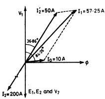
I<sub>2</sub>=200 A;  $\phi_2 = \cos^{-1}0.8 = 36.86^\circ$ ; I<sub>0</sub>=10 A;  $\phi_0 = \cos^{-1}0.1 = 84.26^\circ$ ; I'<sub>2</sub> = I<sub>1</sub>(N<sub>1</sub> / N<sub>2</sub>) = 200(1/4) = 50 A; angle between I<sub>2</sub> and I<sub>0</sub> = 84.26° - 36.86 = 47.4° A.
