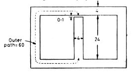
Central limb : Ac = 4cm×4cm =  $1.6 \times 10^{-3}$  m<sup>2</sup> ;  $l_c = 24$  cm =  $2.4 \times 10^{-1}$  m ; B<sub>c</sub> =  $\phi_c/A_c = (1.6 \times 10^{-3} = 1 \text{ Wb/m}^2.$
