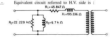
Test data on a single-phase, 250/500 V, 50 Hz transformaer are:
