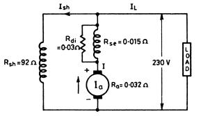
$$I_{sh} = 230/92 = 2.5 \text{ A} \text{ ; } I_{a} = I_{L} + I_{sh} = 150 + 2.5 = 152.5 \Omega.$$
