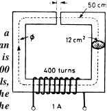
permeability of 1,300. Calculate : (1) reluctance of iron part of the magnetic circuit ; (2) reluctance of the air-gap ; (3) total reluctance ; (4) total flux, and (5) flux density in the air-gap. Neglect leakage and fringing.
