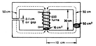
Calculate the exciting current required to produce a flux of 1 mWb in the air-gap. Neglect leakage, and fringing. B/H curve is as follows :
