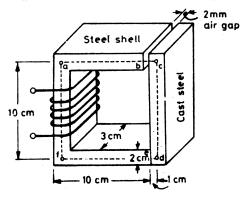
In the above, relay assume that the relay is open so that a 2 mm air-gap is introduced at point b. Find the current to establish a flux of 0.3 mWb in the air-gap.
