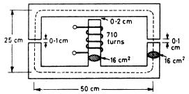
Calculate the current required to produce flux of 1.8 mWb is an air-gap of 0.2 cm length. Magnetising curve for cast iron is :
