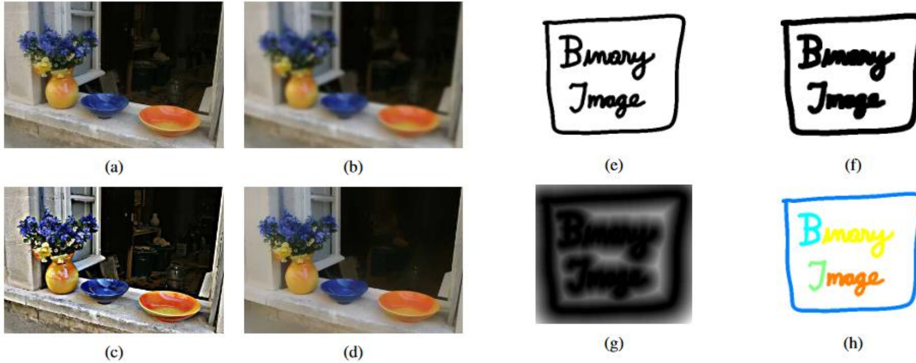
Figure 3.11 Some neighborhood operations: (a) original image; (b) blurred; (c) sharpened; (d) smoothed with edge-preserving filter; (e) binary image; (f) dilated; (g) distance transform; (h) connected components. For the dilation and connected components, black (ink) pixels are assumed to be active, i.e., to have a value of 1 in Equations (3.44–3.48).
