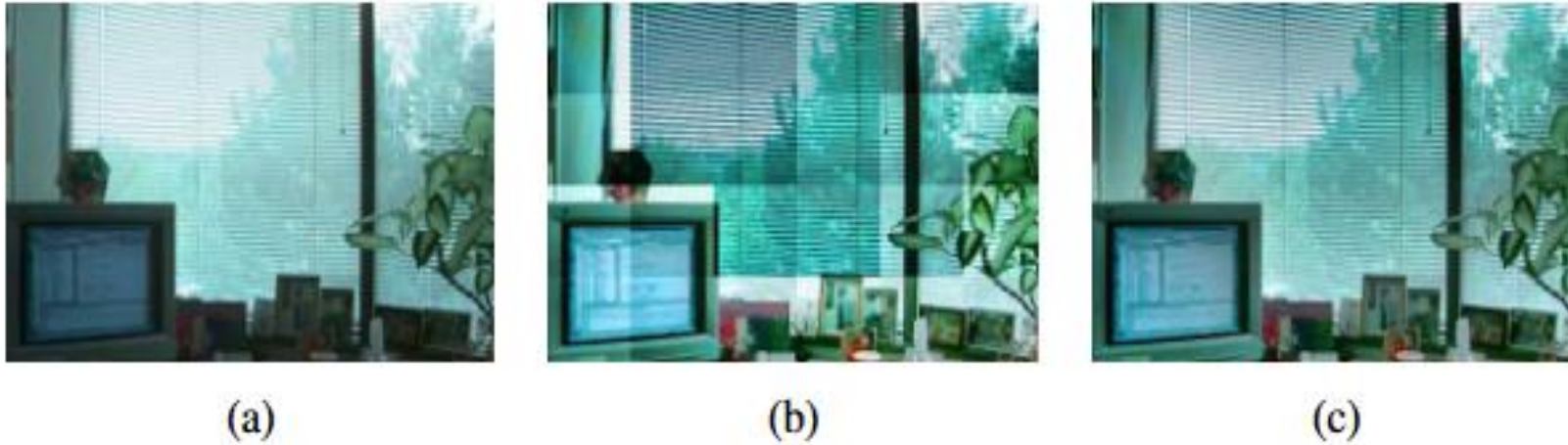
Figure 3.8 Locally adaptive histogram equalization: (a) original image; (b) block histogram equalization; (c) full locally adaptive equalization.
