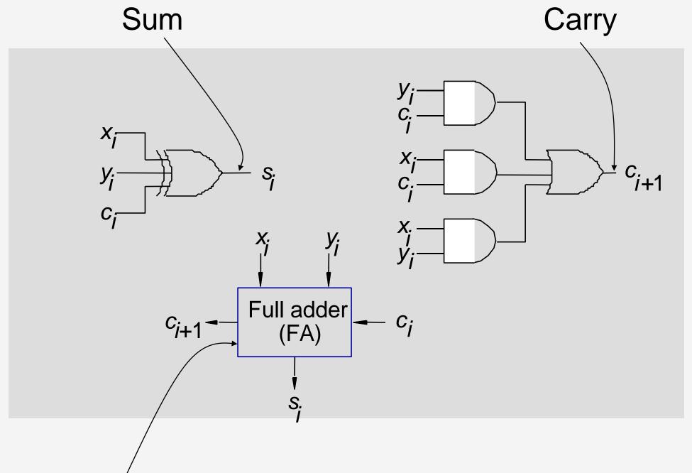
Full Adder (FA): Symbol for the complete circuit for a single stage of addition
