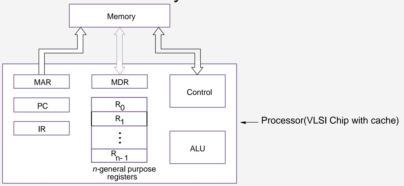
Connections between the processor and the memory.
