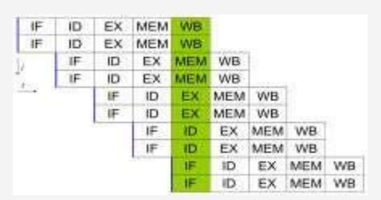
Simple superscalar pipeline. By fetching and dispatching two instructions at a time, a maximum of two instructions per cycle can be completed.
