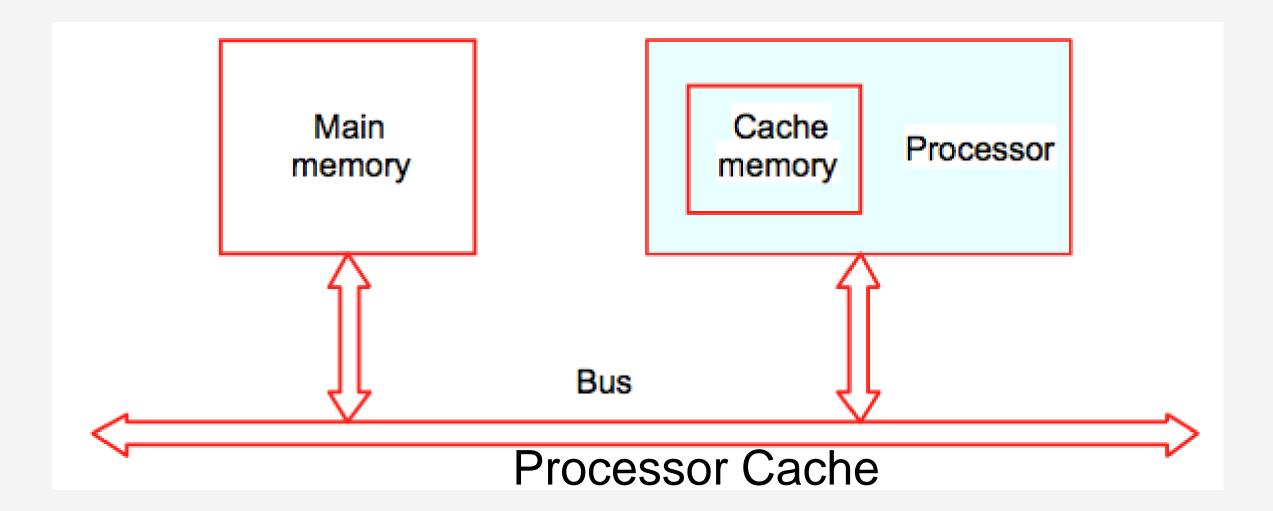
The processor and a relatively small cache memory can be fabricated on a single integrated circuit chip.
