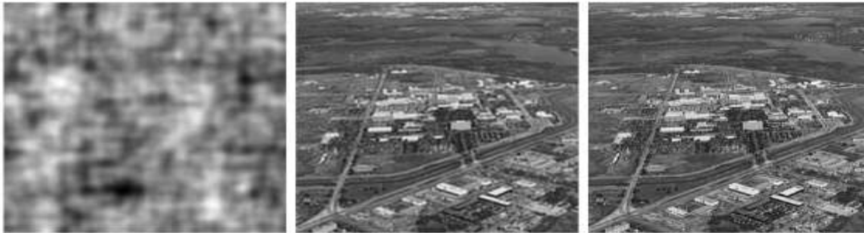
FIGURE 5.28 Comparison of inverse and Wiener filtering. (a) Result of full inverse filtering of Fig. 5.25(b). (b) Radially limited inverse filter result. (c) Wiener filter result.
