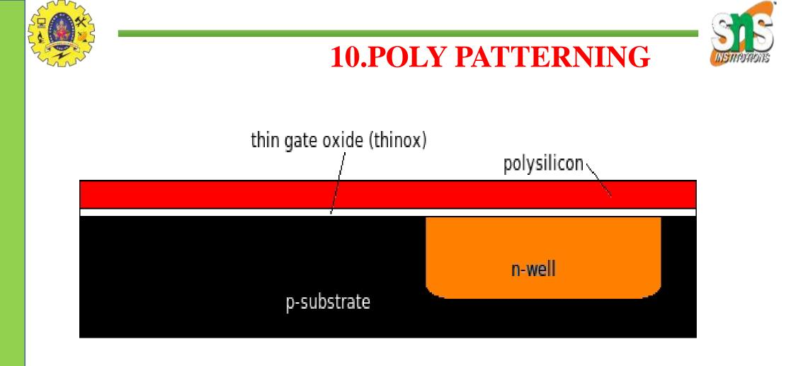
The wafer is now patterned with PhotoResist and the poly maskFinally this leaves the device gates
