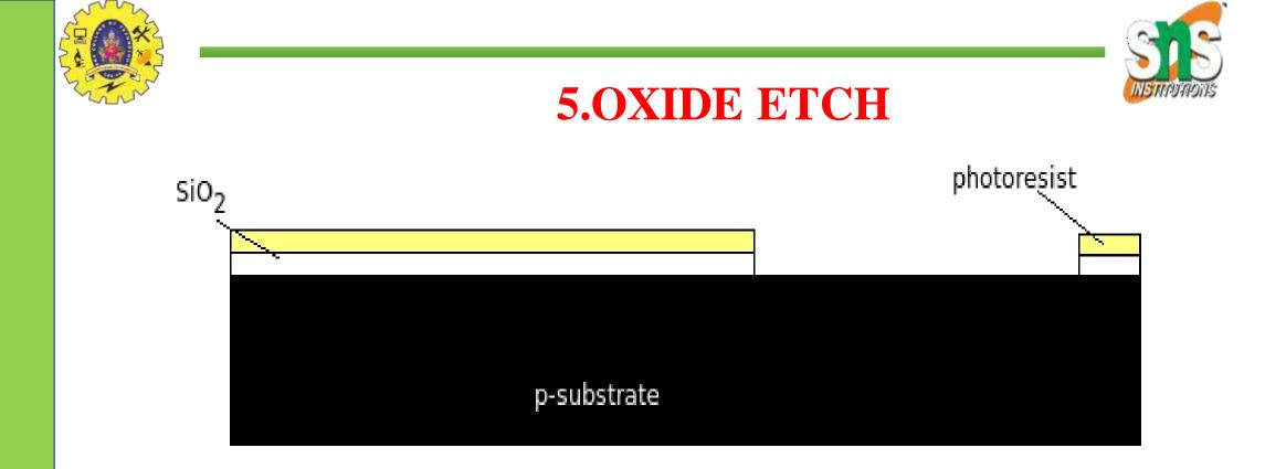
•The oxide is etched with HF acid where unprotected by Photo Resist
