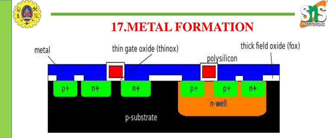
Al is sputtered over the entire area filling contact cuts tooMetal is patterned with the metal mask
