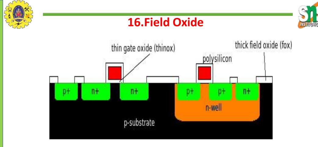
The field oxide is grown to insulate wafer and metalIt is patterned with the contact mask
