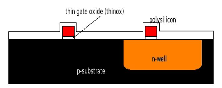
Again, a protective oxide is grown and PhotoResist deposited
