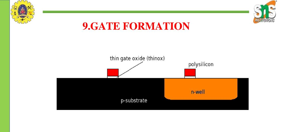
The gates are made up of polysilicon over thinoxCVD is used to grow the poly (heavily doped) layer
