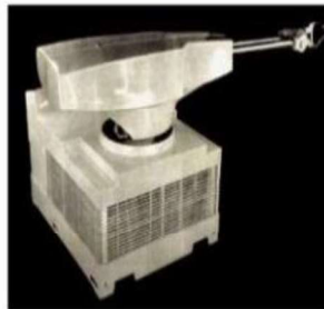
1961 - The first industrial robot was online in a General Motors automobile factory in New Jersey. It was called UNIMATE. It was used to pick up and put down parts.
