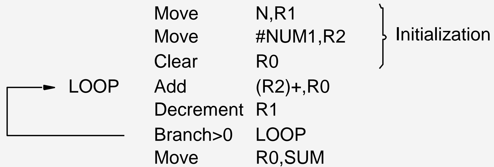
Figure 2.16. The Autoincrement addressing mode used in the program of Figure 2.12.
