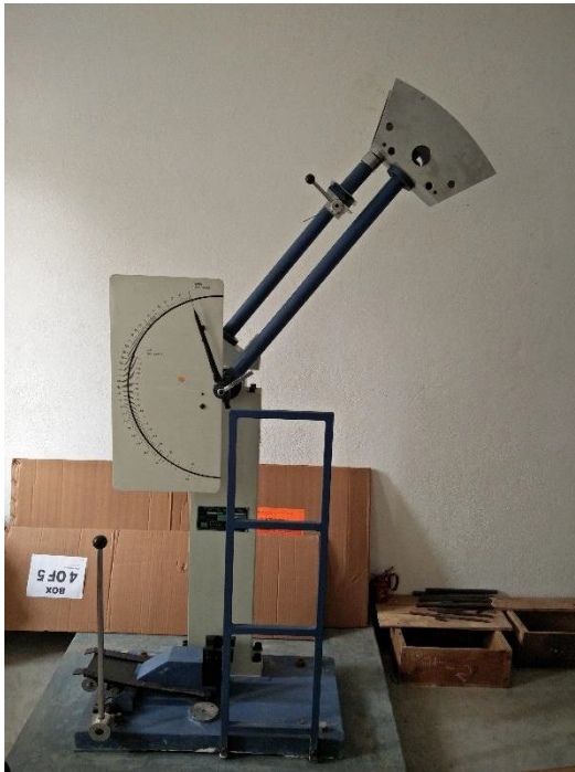
Fig 3.1 Impact test equipment
