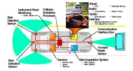
A collision warning system, also known as a Forward Collision Warning (FCW) system, is a safety feature in vehicles designed to alert the driver when it detects a potential collision or imminent danger with a vehicle, object, or pedestrian in the vehicle's path. Here are key points about collision warning systems:
