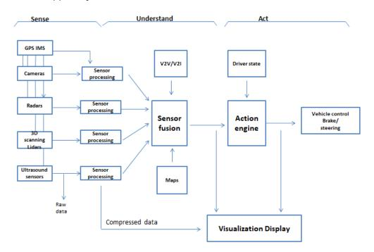
Driver support systems encompass a wide range of technologies and features that assist drivers in various aspects of their driving tasks. These systems are often integrated into modern vehicles
