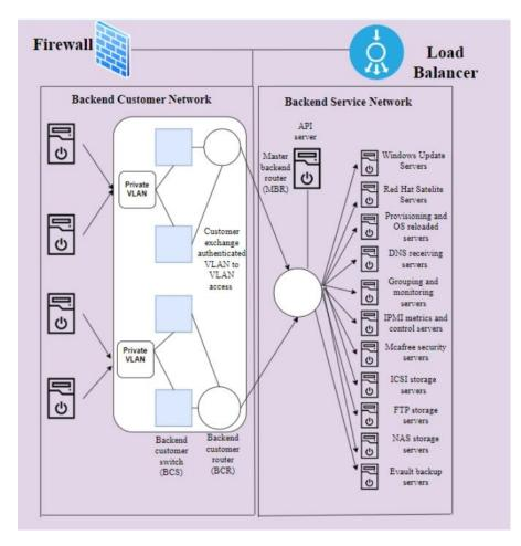
A physical firewall is present at the top of the diagram below.
