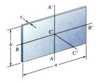
• For the principal centroidal axes on a rectangular plate,  $I_{AA'} = \rho t I_{AA',area} = \rho t \left(\frac{1}{12}a^3b\right) = \frac{1}{12}ma^2$   $I_{BB'} = \rho t I_{BB',area} = \rho t \left(\frac{1}{12}ab^3\right) = \frac{1}{12}mb^2$   $I_{CC'} = I_{AA',mass} + I_{BB',mass} = \frac{1}{12}m\left(a^2 + b^2\right)$
