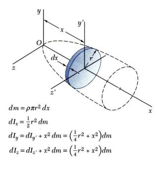
• Moment of inertia of a homogeneous body is obtained from double or triple integrations of the form
