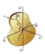
• For the axis *CC*' which is perpendicular to the plate,  $I_{CC'} = \rho t J_{C,area} = \rho t \left( I_{AA',area} + I_{BB',area} \right)$  $= I_{AA'} + I_{BB'}$
