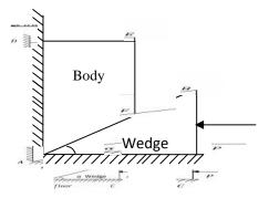
A wedge is a piece of wood or metal, usually of a triangular or trapezoidal in cross-section, used for lifting loads or for slight adjustments like tightening keys for shafts.
