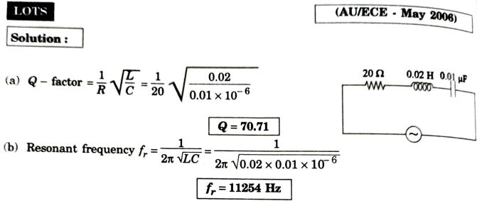
**EXAMPLE 20:** Determine the resonant frequency for the circuit.
