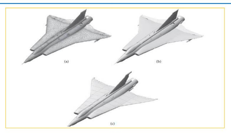
(a) Wireframe polygonal model (b) Polygonal surface model
